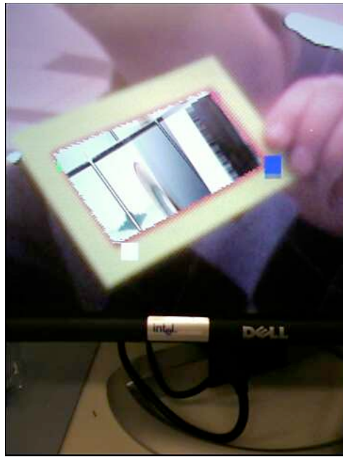
Figure 8: A photo of the final system image showing interpolation error. The grid interpolation module successfully maintains rotations and scaling, but fails to properly fit the image on to the card. This is likely due to an overflow of an intermediate value in the processing chain.
