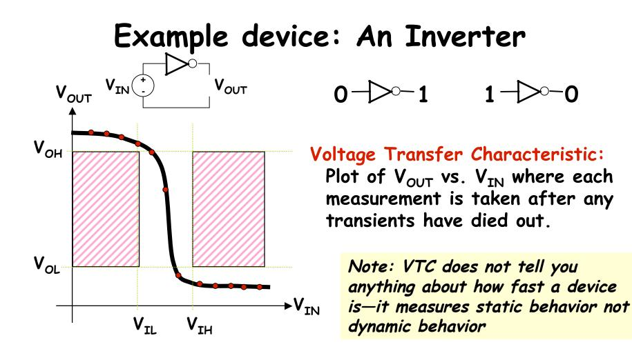
Static Discipline requires that we avoid the shaded regions aka "forbidden zones"), which correspond to valid inputs but invalid outputs. Net result: combinational devices must have GAIN > 1 and be NONLINEAR.
