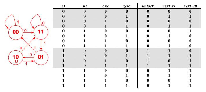
B. (10 Points) What's the N-digit combination for the lock, i.e., what sequence of 0's and 1's will leave you with UNLOCK asserted regardless of what state the FSM was in when you started to enter the combination? Hint: use the truth table to draw a state transition diagram. You can use the back of the quiz pages as scratch paper.
