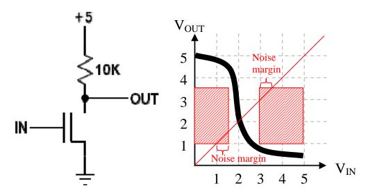
A. (10 Points) Choose values for  $V_{OL}$ ,  $V_{IL}$ ,  $V_{IH}$  and  $V_{OH}$  so that the prototype device obeys the static discipline and has positive, non-zero noise margins. Give your values below or briefly explain why no such values can be found.
