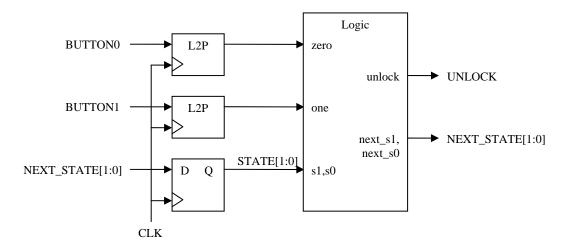
A. (10 Points) The L2P module is a level-to-pulse converter that asserts its output high for 1 clock cycle after a 0-to-1 transition on its input, as shown in the timing diagram below.
