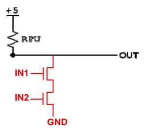
C. (5 Points) Assume that all mosfets in Hot Logic's gates have the same width and length. If we want the  $V_{OL}$  for the HL-NAND gate to be the same as the  $V_{OL}$  for the HL-INV gate, what value should we choose for RPU?
