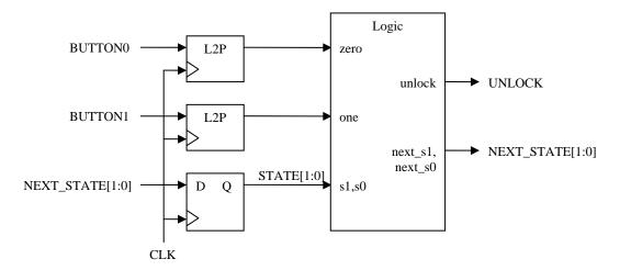
A. (10 Points) The L2P module is a level-to-pulse converter that asserts its output high for 1 clock cycle after a 0-to-1 transition on its input, as shown in the timing diagram below.
