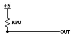
C. (5 Points) Assume that all mosfets in Hot Logic's gates have the same width and length. If we want the  $V_{OL}$  for the HL-NAND gate to be the same as the  $V_{OL}$  for the HL-INV gate, what value should we choose for RPU?
