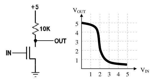
A. (10 Points) Choose values for V<sub>OL</sub>, V<sub>IL</sub>, V<sub>IH</sub> and V<sub>OH</sub> so that the prototype device obeys the static discipline and has positive, non-zero noise margins. Give your values below or briefly explain why no such values can be found.
