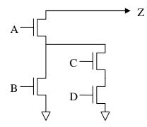
(A) (10 points) Please draw the schematic for the pullup circuitry that correctly completes the implementation of the CMOS gate.
