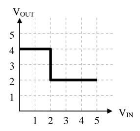
III would like for their devices to have the largest possible noise margins. Please specify choices for  $V_{OL}$ ,  $V_{IL}$ ,  $V_{IH}$  and  $V_{OH}$  that meet this goal, or briefly explain why devices with the given voltage transfer curve can't be used as combinational devices with positive noise margins.
