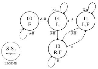
(A) (16 Points) Please <u>neatly</u> fill in the truth table for the FSM's combinational logic below: using S<sub>1</sub>, S<sub>0</sub>, A and B as the inputs, and using next\_S<sub>1</sub>, next\_S<sub>0</sub>, F, L and R as the outputs.
