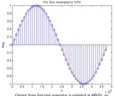
Output from function generator is sampled at 48kHz, so to create different frequencies, a 48000/N Hz sine function is sampled at N/f points, where N is the number of samples and f is the desired frequency.
