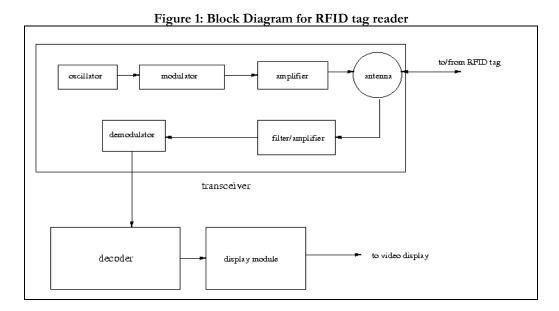
The transceiver's antenna will include a 125 kHz transmitter with low distortion for interrogation of tags, and a 62.5 kHz receiver to get the reply. Since the tag will send its data as an amplitude modulated (AM) signal, the reader will filter the signal to select and amplify the 62.5 kHz carrier, and demodulate it to get the signal transmitted by the tag. When it is done, it will flash a green LED to indicate successful reception.
