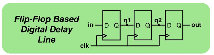
Will nonblocking and blocking assignments both produce the desired result?
