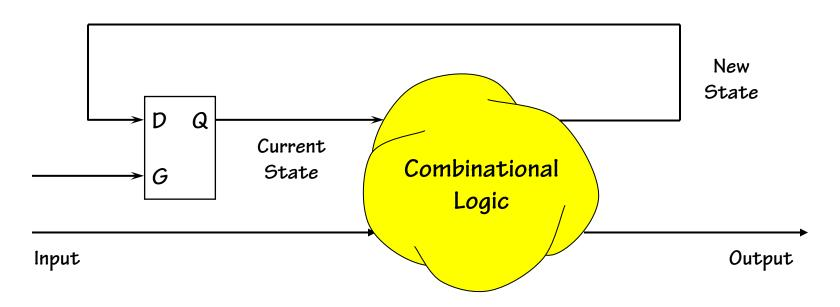
Plan: Build a Sequential Circuit with one bit of STATE -
