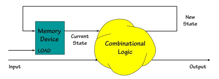
Plan: Build a Sequential Circuit with stored digital STATE -
