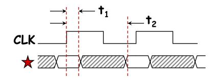
$$t_1 = t_{CD,reg1} + t_{CD,1} > t_{HOLD,reg2}$$
