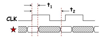
$$t_1 = t_{CD,reg1} + t_{CD,1} > t_{HOLD,reg2}$$
