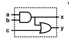
module blocking(a,b,c,x,y); input a,b,c; output x,y; reg x,y; always @ (a or b or c) begin x = a & b; y = x | c; end
