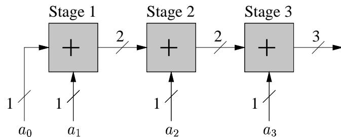
Each stage  $i$  of this circuit adds the bit  $a_i$  into a running sum, which it forwards to stage  $i + 1$ . Each cable of wires in the figure is labeled with the number of its constituent wires.
