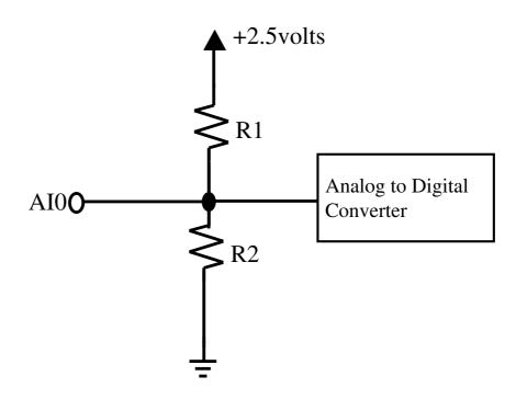
Your task will be to experiment with the NI box and try to determine which input circuit is correct, and to determine the value of any unknown resistors. The tests you performed above will certainly be helpful, but you will need to run additional experiments. Ask the staff if you need resistors. As a handy reference, here is the chart of resistor band colors:
