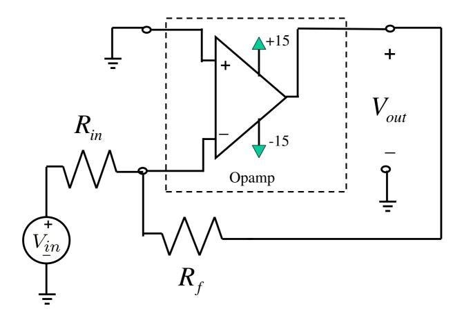
In order to simplify the analysis of the op-amp circuit, we assumed that  $V_+ - V_- \approx 0$  and that no current enters the op-amp inputs. Using those assumptions, we determined that the relationship between  $V_{in}$  and  $V_{out}$  was
