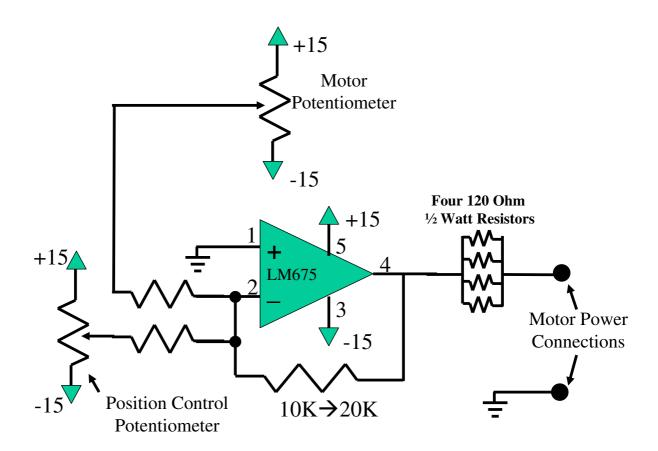
Motor Driver Circuit - Unmarked Resistors are 10k ohms
