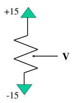
When the potentiometer is used to create a voltage divider, the resistors in the divider are related to head angle  $\theta$ , see below, and so the voltage produced will be proportional to the head angle.
