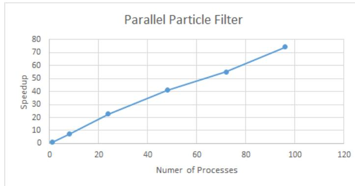
Figure 7: Graph showing the speedup as we parallelize across multiple machines
